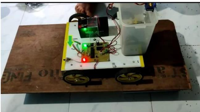
The path hole will be detected with the help of ultrasonic sensor. The sensors will continuously transmit an ultrasonic wave from the transmitter and then wave will travel in air and reflect back to the sensor’s receiver. If there is any disturbance or differences between transmitted and received wave (i.e. if pulse width is more than 25ms), the microcontroller will detect the Pothole and the machine will stop.
