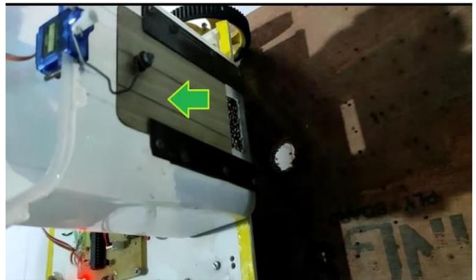
The output shaft of the servomotor is capable of traveling somewhere around 180 degree. A 1.5ms pulse is provided to servomotor which makes the motor turn 90-degree position, which lifts the slat and thus allows material to fall on detected pothole.
