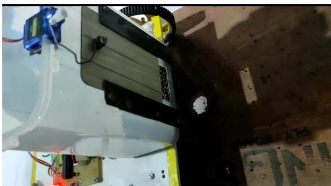
After dumping the material in pothole, the model will again move backward and will check whether the hole is filled completely in the same way as it did in step 2. If it is not filled completely it will again repeat step 3 and 4. Or else it will move forward.
